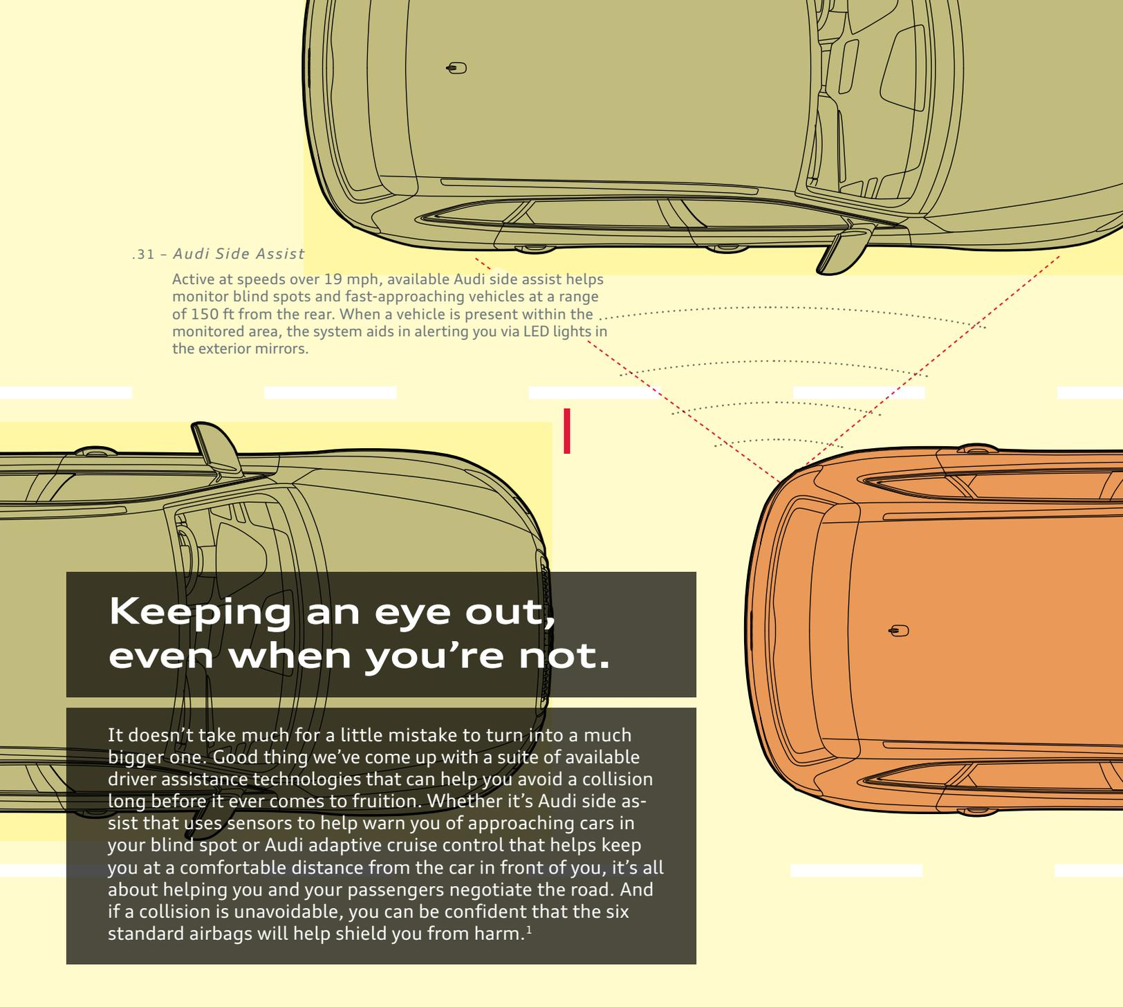
A diagram illustrating the Audi Side Assist system. It shows a top-down view of a car with a sensor on the roof. Dotted lines represent the sensor's range, which is wider on the side than in front or back. A red dashed line indicates the sensor's field of view. A vertical red line is positioned between the car and a second car on the right. The background is yellow with white dashed lines representing lane markings.
